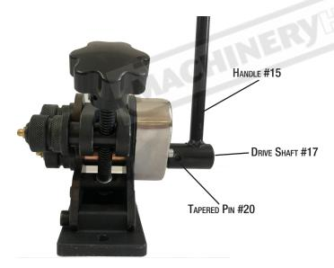
2. Secure the Handle (15#) to the Drive Shaft (17#) using the Taper Pin (20#). Insert the Taper Pin (20#) into the hole as seen in the Figure above. If necessary, lightly tap the Taper Pin (20#) into place.
